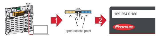
Establish a connection to the inverter (LAN1) with a network cable (CAT5 STP or higher).
