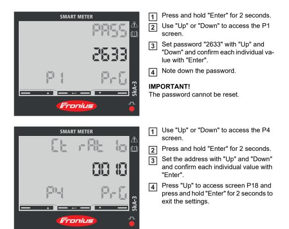
Ratio of current transformers<sup>1)</sup> (0001 -  $1000^{2}$ ). Ratio of voltage transformers<sup>1), 3)</sup> (001.0 -  $1000^{2}$ ).
