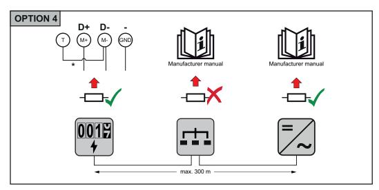
\* The terminating resistor for the Fronius Smart Meter TS is manufactured with a wire between  ${\bf M}$  and  ${\bf T}.$
