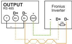
\* To avoid interference, the terminating resistor must be used (see chapter **Terminating resistors** on page **23**). This is integrated in the Fronius Smart Meter TS and must be manufactured with a wire between **M** and T(T = termination).
