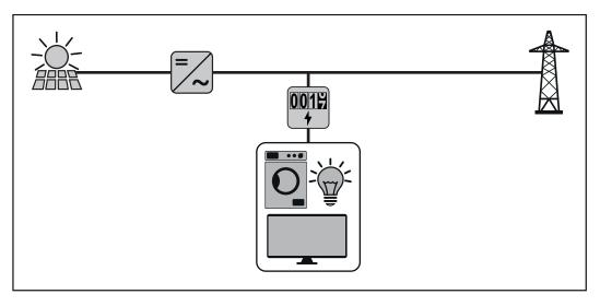
For use as a secondary meter to measure individual loads and producers, see chapter **Multi-meter system** on page **25**.
