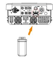
For the -P/-E version of Pocket WiFi. screw the antenna to the end of the shell
