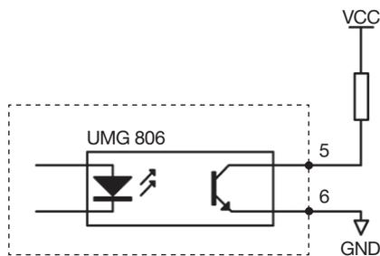
Fig.: Schematic diagram of digital output
