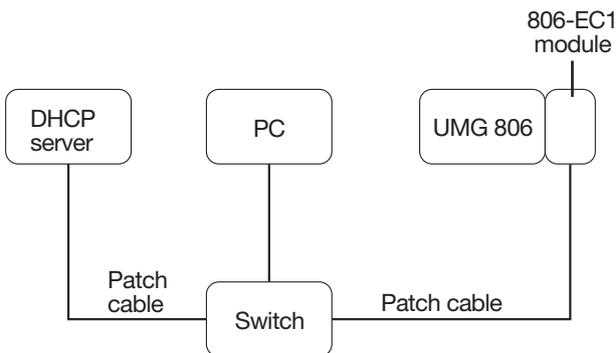
*Fig. Connection example: UMG 806 with 806-EC1 module and PC are automatically assigned the IP address by a DHCP server (parameter 205 = 1 - default setting).*
