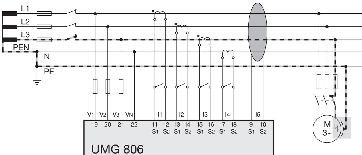
Fig. Connection example, UMG 806 with residual current monitoring
