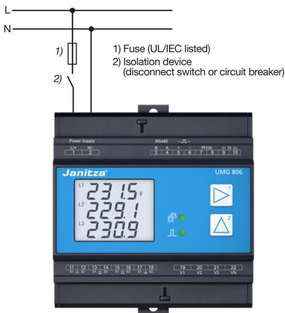
Fig. Supply voltage connection.
