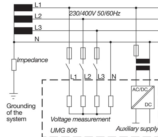
Fig. Schematic diagram, UMG 806 in an IT network with N.
