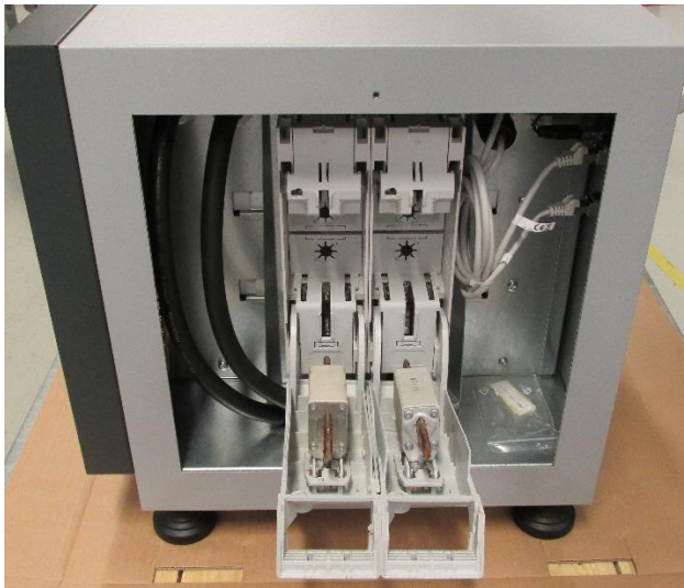
Figure 4-13: battery storage system, side view, power isolator pulled
