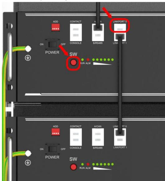
5) Press the **red SW button of master battery** to power on, all the battery LED light will be on one by one from the Master battery:
