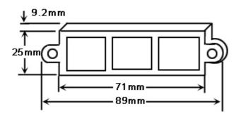
Voltage : 24 V/DC Resistance : 9.5 ~ 18.5 ohm Current : 5 ~ 6 A Power (max.) : 130 W Surface temperature (max.) : 240 ° C
