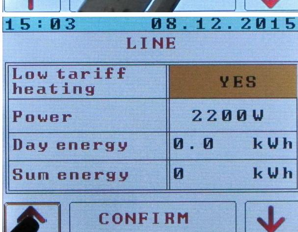
LINE screen allows setting of usage of mains energy - we can select to use mains energy only during low tariff. It also shows information about used mains energy (day and overall).
