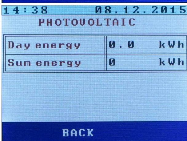
PHOTOVOLTAIC screen shows information about electricity production by PV panels: Day production (Day energy) and overall production (Sum energy). Values can be deleted, as well as in the line menu.
