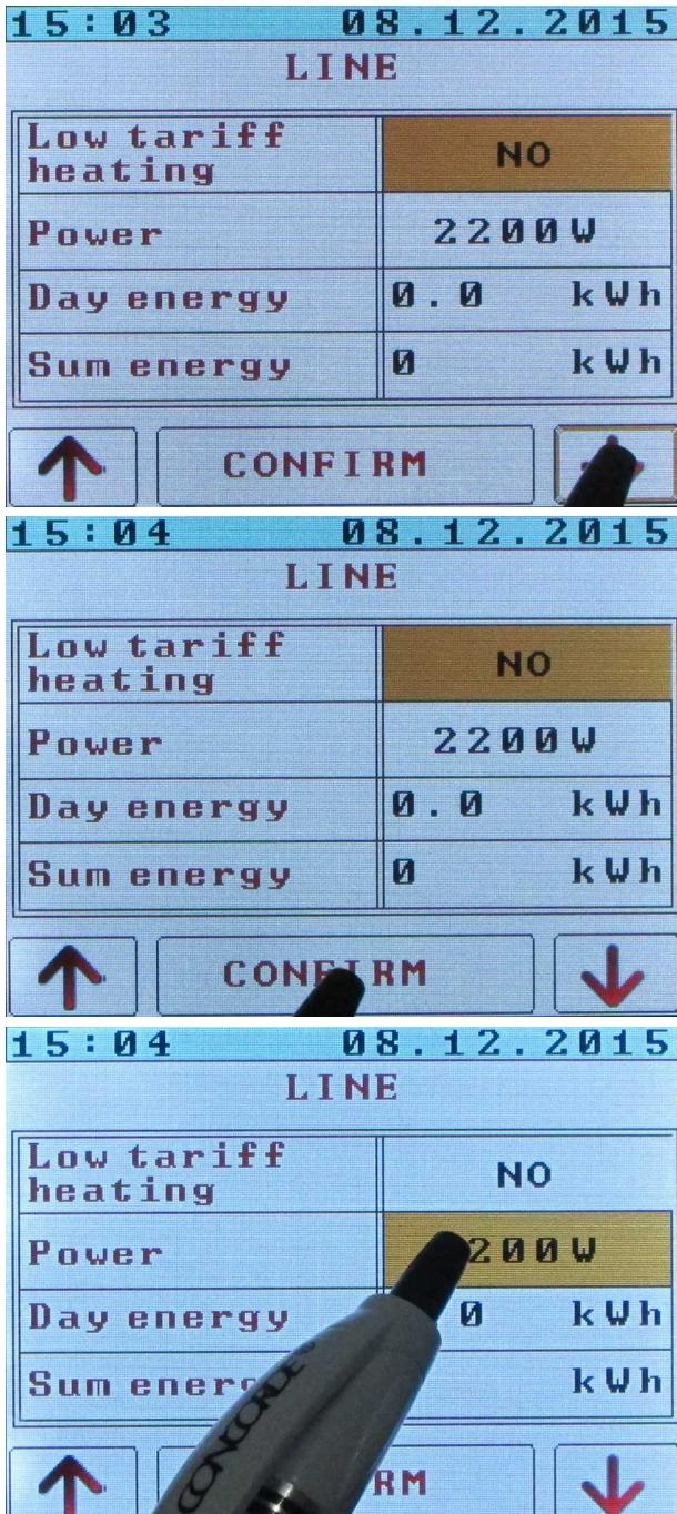
Pressing arrow DOWN activates mode, when boiler can use mains energy anytime he needs.
