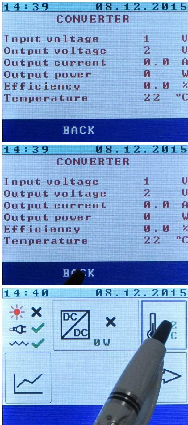
CONVERTER MENU screen shows information of converter status - input voltage, output voltage, output current, output power, actual efficiency and temperature inside of a heating element.
