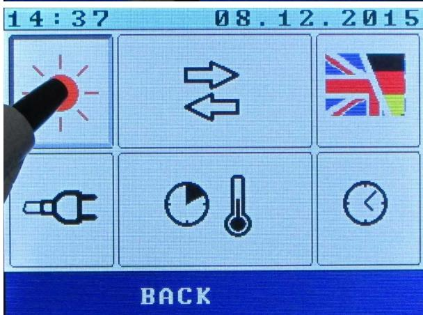
By pressing an icon of solar panel, PHOTOVOLTAIC menu is opened.
