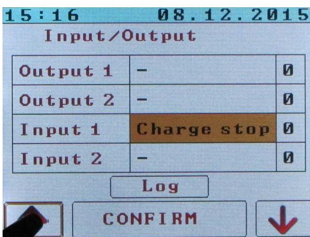
Select the required switching condition by pressing up/down arrow. This function serves to stop the chosen method of heating and thus to prioritize a different course with regard to the setting temperature. From a practical point of view it makes sense to primarily supply AC Stop heating, which prefer the DC heater, for example if the available another source of heating and we do not want heat the water with mains power.
