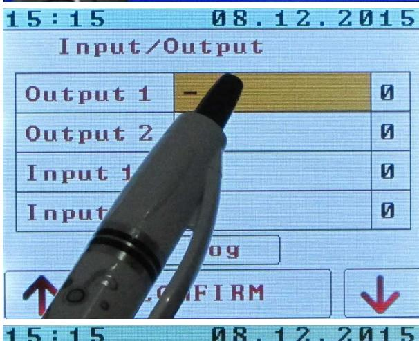
Touching to the table allows edit value. In the input/output menu left column contains the name, the middle column is an optional condition activation of the input/output, and the right column of his current status.
