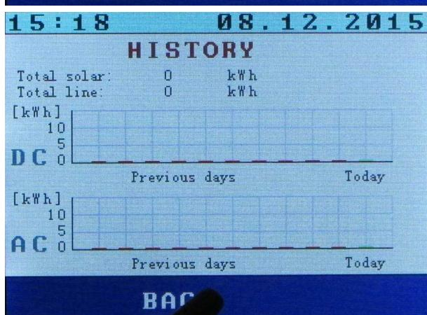
Press the chart symbol to open the informative display of the power consumption in the last days.
