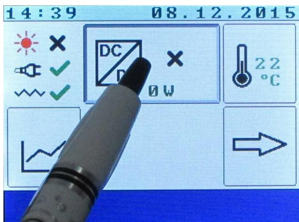
By pressing an icon of a converter, CONVERTER MENU is opened.
