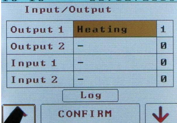
Select the required switching condition by pressing up/down arrow.
