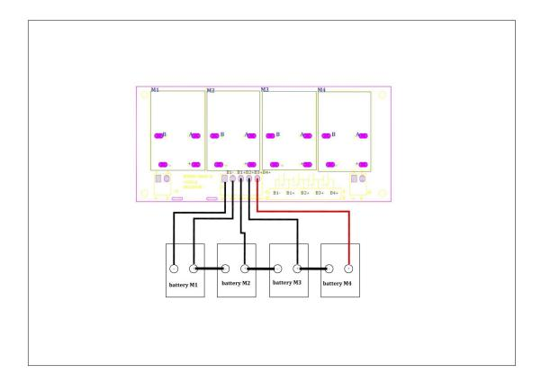
All the balancers are connected to the batteries in parallel.
