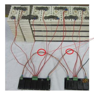
the wires between each balance modules are called "balance wires".
