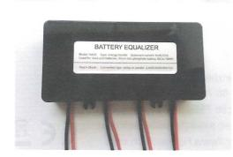
HA02 battery equalizer is energy transfer type equalizer, it can compensate for batteries with two sides. The equalizer starts to work when there are 10mV between t wo batteries. The current will flow from a higher voltage to low voltage, eventually reach equilibrium. It can connect with battery system with 24 hours, to keep the system energy balance automatically, no need manual maintenance.
