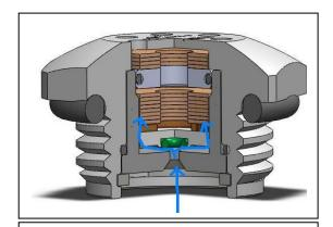
Water entering the valve from the radiator expands the hygroscopic washers.
