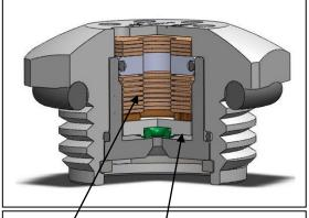
The expanded washers close the valve by pushing the plastic washer containing a viton seal against the inlet port.
