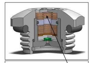
At the end of valve life the top safety washers expand and close the valve permanently.
