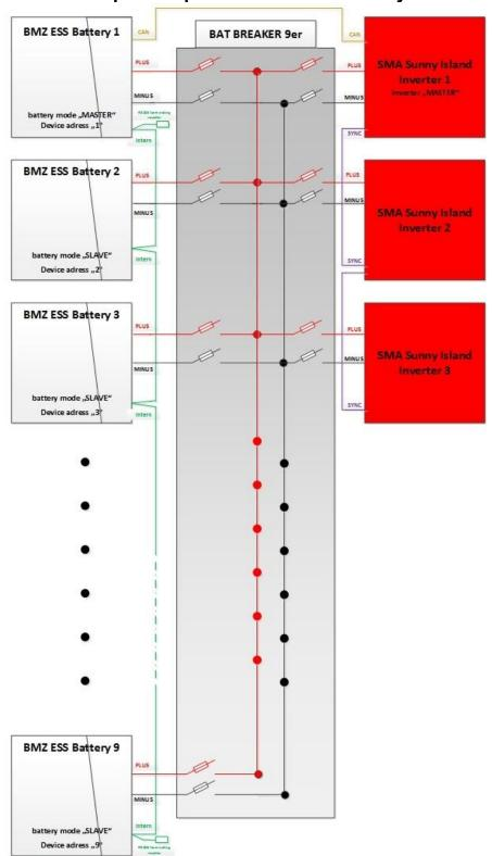
Figure 4-25: 3-phase operation on 9 ESS batteries
