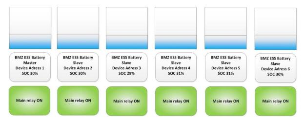
Figure 4-38: representation of example 3, different SOC of BMZ ESS batteries connected in parallel
