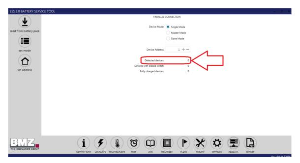
Figure 4-39: check the number of BMZ ESS batteries connected in parallel
