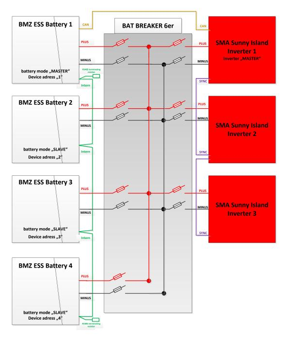
Figure 4-22: 3-phase operation on 4 ESS batteries
