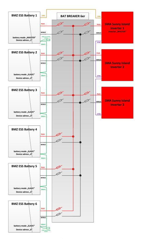
Figure 4-24: 3-phase operation on 6 ESS batteries
