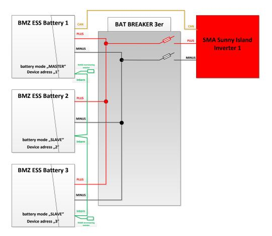
Figure 4-20: 1-phase operation on 3 ESS batteries
