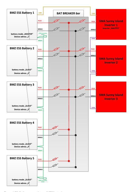
Figure 4-23: 3-phase operation on 5 ESS batteries
