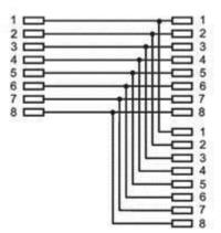
Figure 4-12: pin assignment of RJ45 Y-adapter (T-connector)
