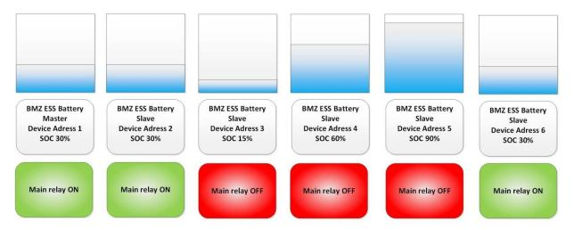
Figure 4-36: representation of example 1, different SOC of BMZ ESS batteries connected in parallel
