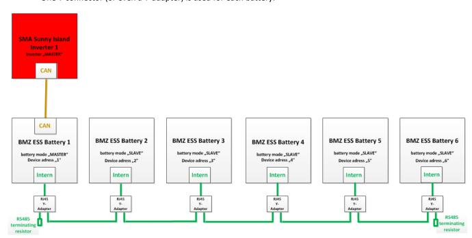
Figure 4-10: communication cabling, ESS parallel connection
