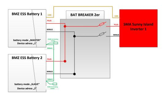
Figure 4-19: 1-phase operation on 2 ESS batteries
