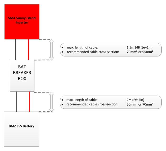
Figure 4-14: cable lengths of the ESS system
