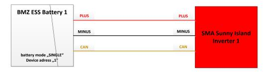
Figure 4-18: 1-phase operation on 1 ESS battery
