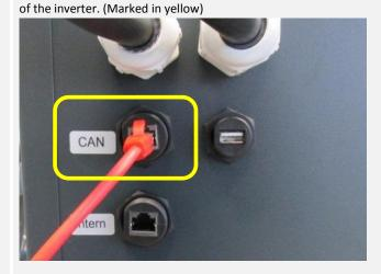
Figure 4-6: representation of external connections of the battery system, CAN
