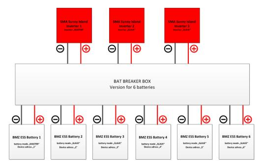
Figure 4-15: output cable of BAT Breaker Box
