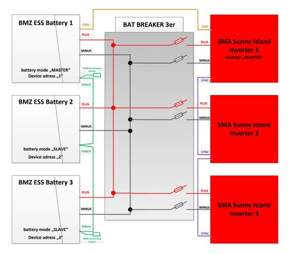
Figure 4-21: 3-phase operation on 3 ESS batteries
