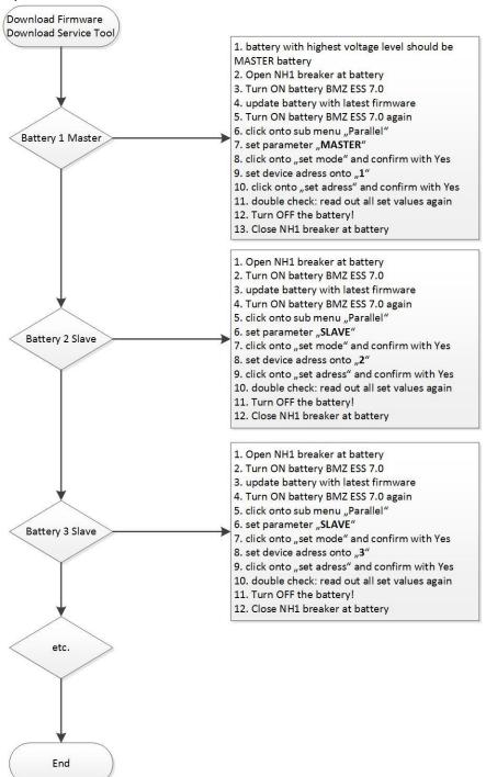
Figure 4-28: representation of the work sequence to configure the parameters of a BMZ ESS battery
