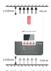
Fig. 2.1 Installation and heat dissipation
