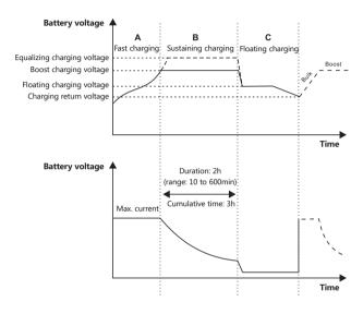
Fig. 1-5 Battery charging stages diagram
