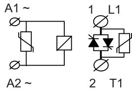
In AC controlled types only (RG..A..) a varistor is placed across A1/A2 terminals.
