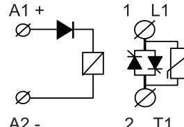
In DC controlled types only (RG..D..) a diode is placed in series with the control circuit for protection against reverse biased connection.
