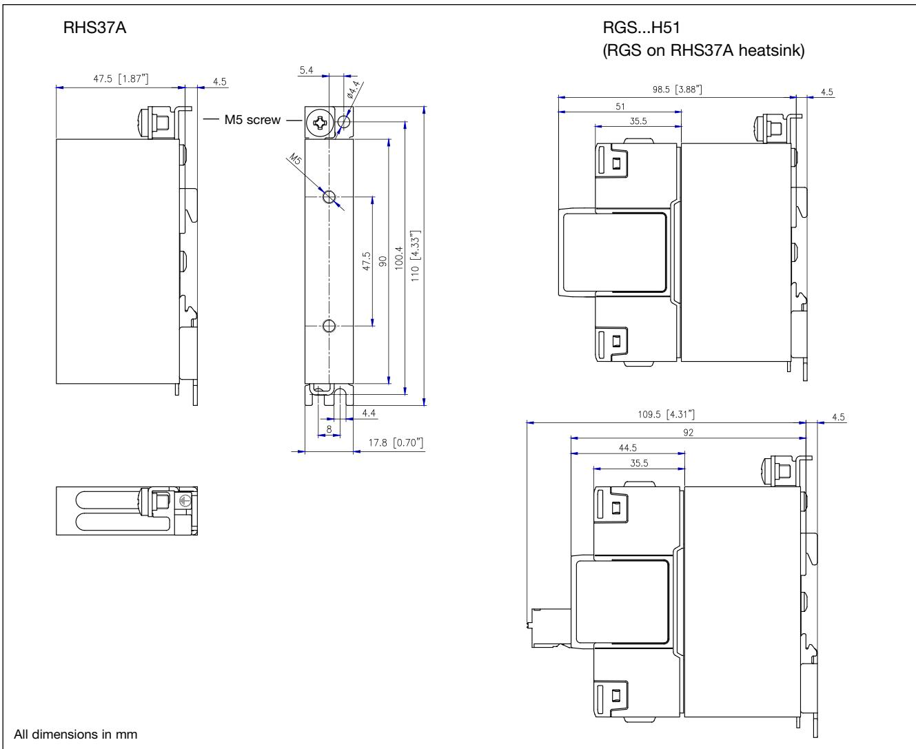
Note: M5 PE screw not provided with SSR. Maximum mounting torque 1.5Nm (13.3 in-lb).
