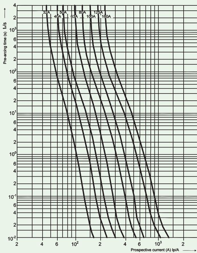
gPV, PV(gR) 750V, 1000V t-l characteristics
