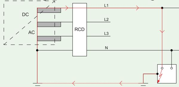
EFI type A can be used in DC/AC inverters with transformers or in DC/AC inverters for which the producer excludes the possibility of DC leakage currents on AC side.
