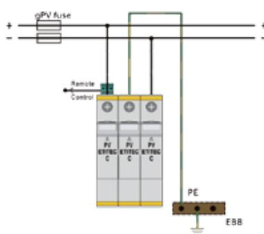
T connection ETITEC C T2 PV
