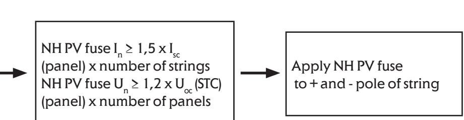
Derating factor 1,5 is defined for ambient temperature max. 45 °C
