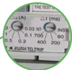
Adjustable residual current tripping thresholds between 30mA and 3A. Adjustable time delay for residual current protection between 60ms and 700ms including INST (instantaneous) and NT (No Trip).
