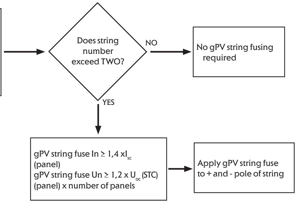
Derating factor 1,4 is defined for ambient temperature max. 45 °C.
