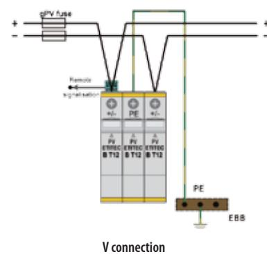
Note: If distance between string and inverter is less than 10 m, then you need only one ETITEC BT12 PV.
